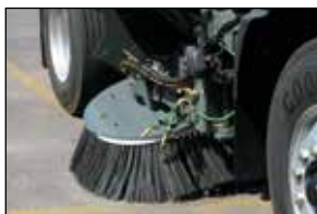
In-cab side broom tilt and extended reach
